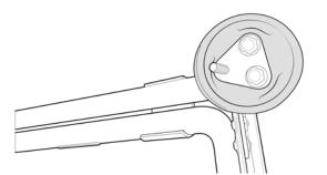
Note - Left hand rear bracket has provision for brake light wire.
