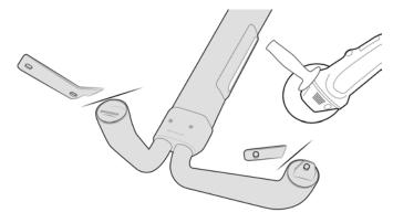
Cut the rear leg as shown be careful not to damage the sports bar.
