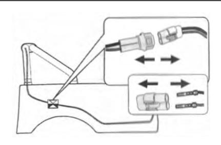
Locate brake light wiring loom from rear passenger side wheel arch. Disconnect and remove plug from connectors.
