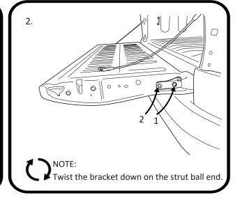
Heavy duty loctite has been used on the indicated bolts from factory. Heating the thread or using rattle gun with a correct phillips head bit will be required.
