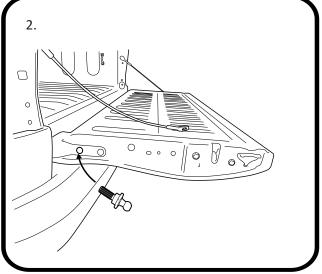
Heavy duty loctite has been used on the indicated bolts from factory. Heating the thread or using rattle gun with a correct phillips head bit will be required.
