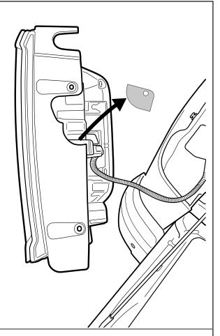
Using stud Ball M6, part number TA-26, fasten to indicated location.
