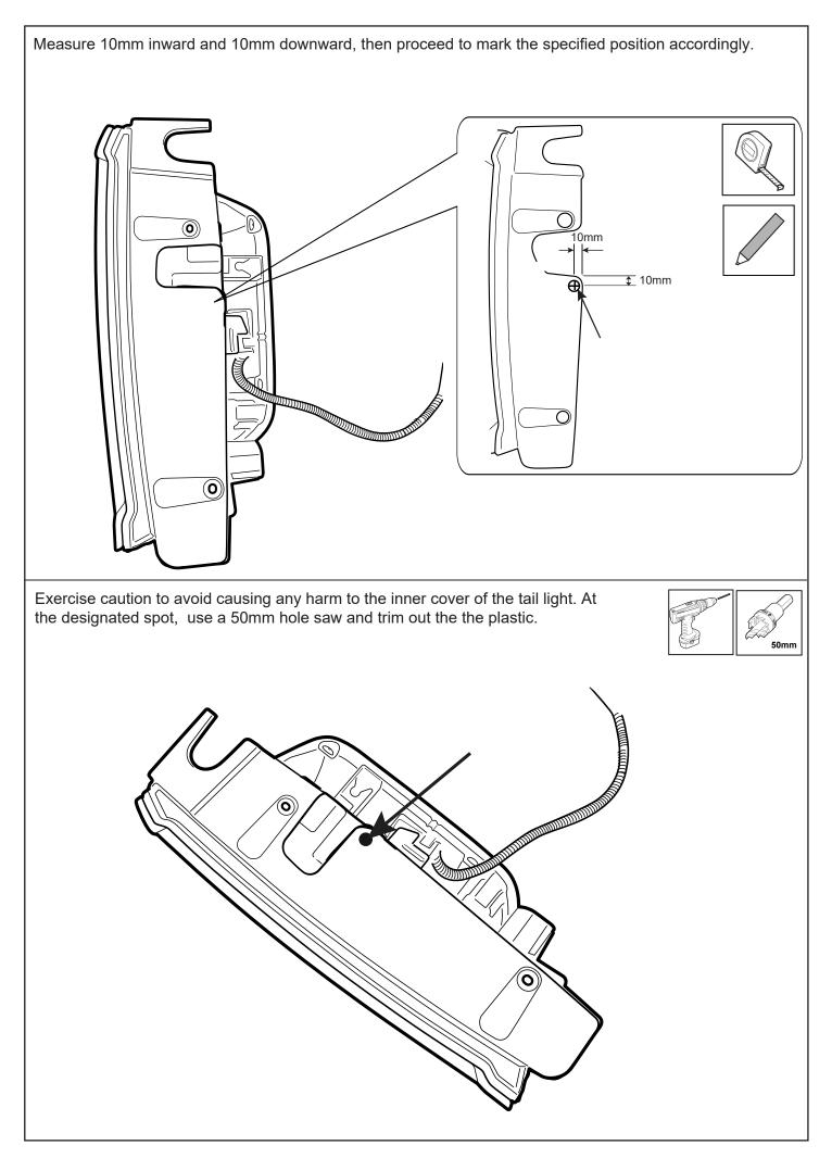
Discard trimmed section and refit the tail light to the vehicle.
